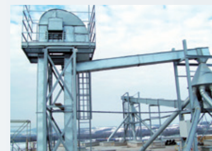
Product distributor comprising belt bucket elevator, chain conveyor and revolving tube distributor
