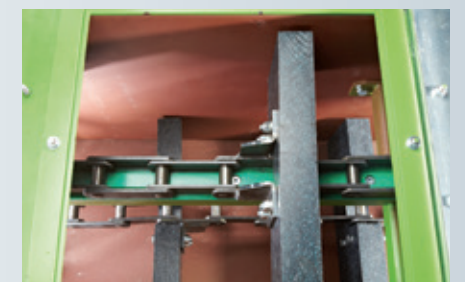
Bushing conveyor chain with screwed plastic tracks
